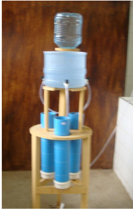
Figure 2. Set up utilized for mobility tests with three plastic columns filled with soil and bentonite.
