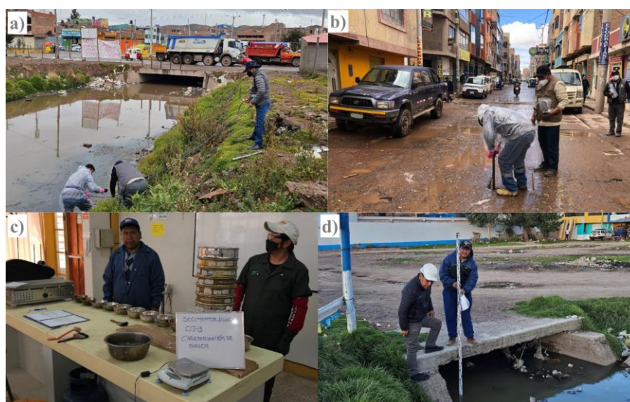
Figure 3. a) Sediment sampling at point DJ3; b) closed-duct sampling; c) laboratory analysis of samples; and d) direct measurement of geometric characteristics of drains.
