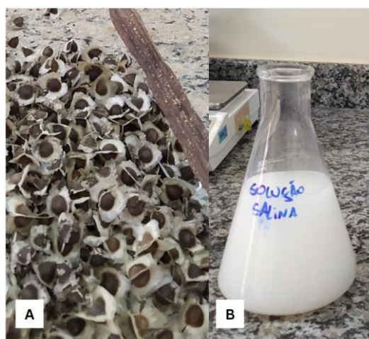
Figure 1. Moringa oleifera coagulant solution - A: seeds and B: saline solution.
