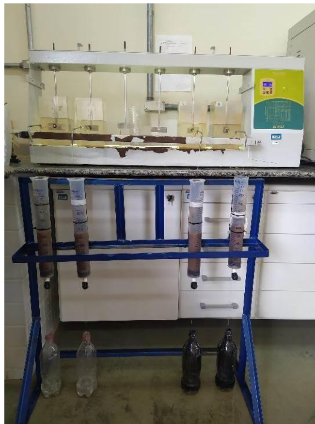
Figure 3. Jar-test equipment associated with filters.
