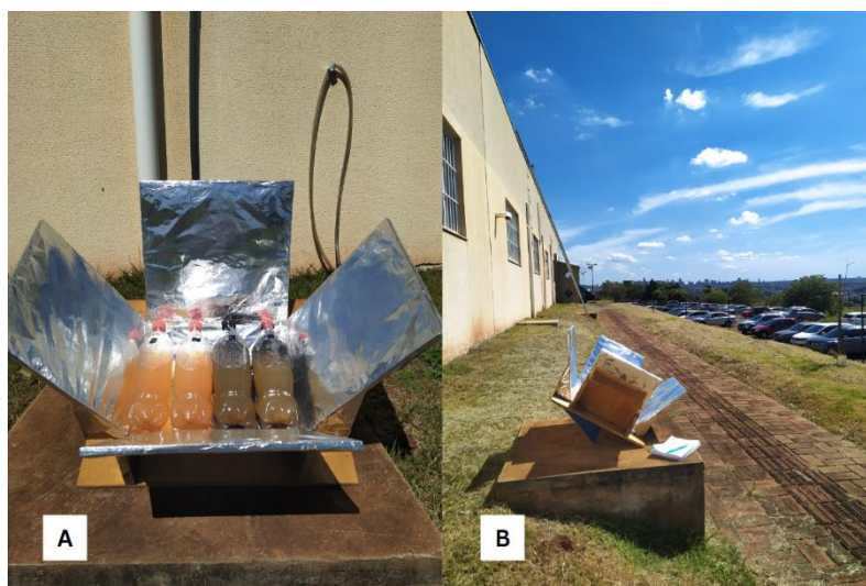
Figure 4. SODIS test (A- Arrangement of the solar concentrator; B- Exposure of the concentrator to the open air).
