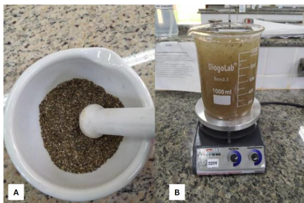
Figure 2. Salvia hispanica coagulant solution – A: seeds in the mortar and B: solution in the magnetic stirrer.
