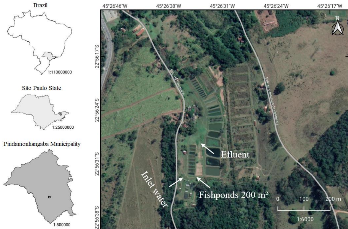
Figure 1. Study area location. The 200 \text{m}^2 excavated fishponds distributed in series, the source of water supply and the place where the effluent is discharged from the fishponds are highlighted. (Google Earth pro source - Image taken on July 23, 2019).
