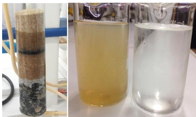
Figure 2. Implanted adsorption system and its result.
