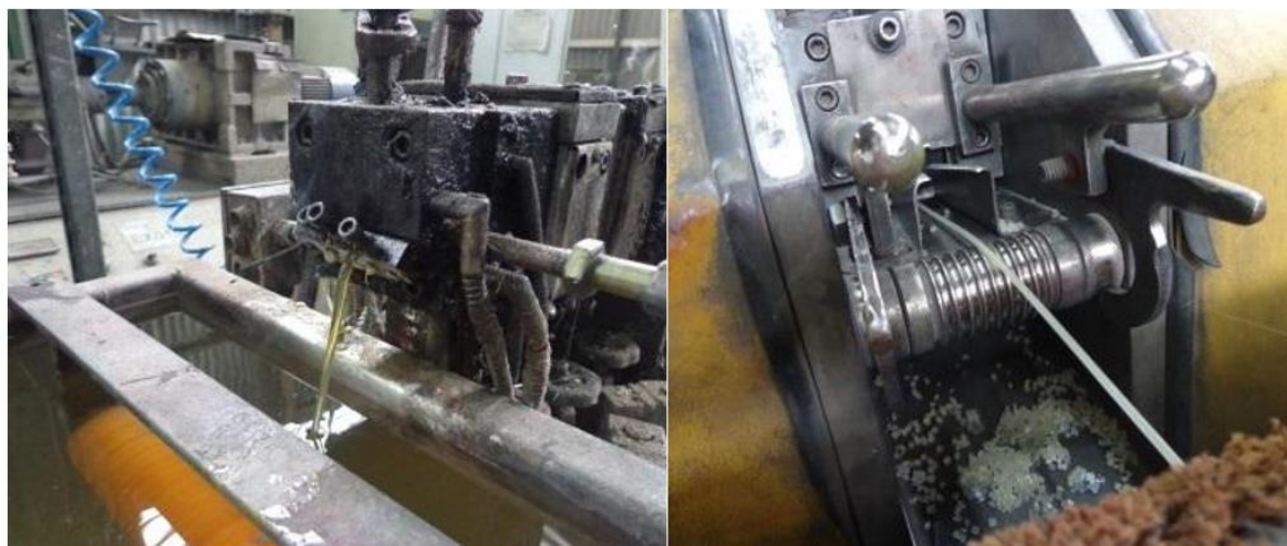
Figure 1. (a) Extruder used to obtain PA/AgNPs filaments; (b) Granulator used to obtain PA/AgNPs pellets.
