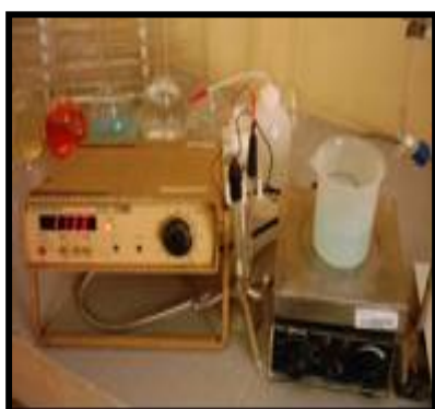
Figure 1. A set up for the potentiometric determination of copper using mercury electrode.
