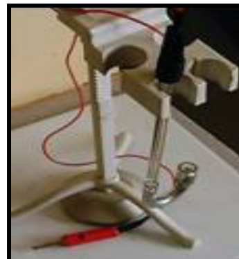
Figure 3. Close up of mercury electrode specially fabricated for this work.
